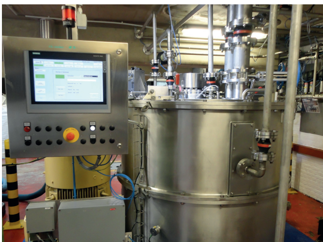
Heinkel Centrifuge V 1250 BC, product contacted parts made of stainless steel (1.4571), with SIEMENS PLC and HMI (Photo: Heinkel)
